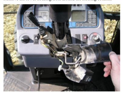
7. Remove the ether switch from the lower housing.
