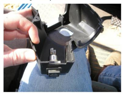
3. Reinstall the lower plastic housing and then reattach the ether switch two-prong connector.
