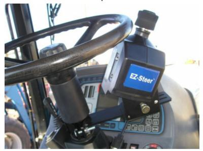
4. Adjust the motor position so there is approximately 2.5–3.2 cm (1-1.25 inches) between the motor drive wheel and the steering wheel ring.
