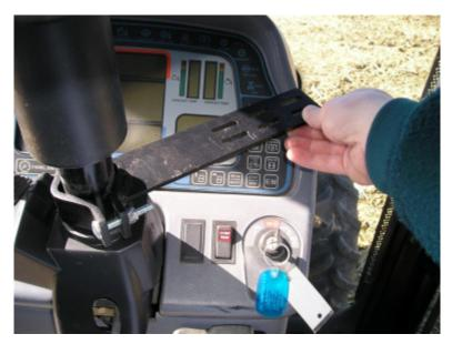
4. Tighten the bracket bolts to 4.1 Nm (3 ft-lbs) torque Use a ½ inch deep socket.
