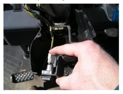
4. Reinstall the two lower screws in the plastic housings.
