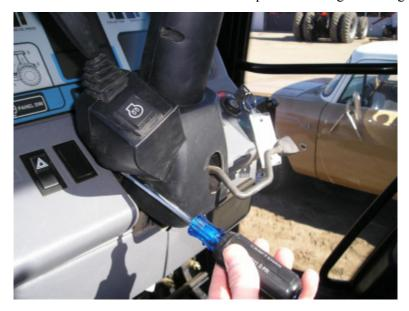
5. Remove the two-prong connector from the ether switch.
