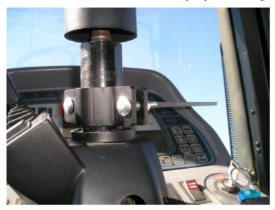
2. Squeeze the bracket clamps together. Use a ½ gear ratchet combination wrench to turn the nuts down against the clamp.
