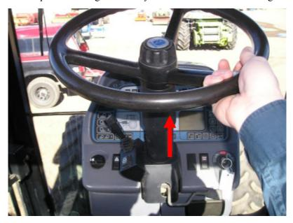
3. Remove the top two screws from the plastic housings covering the steering column.
