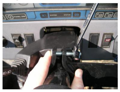
3. Rotate the bracket slotted arm to a 2 o'clock position. Ensure that the end of the bracket will not contact the dash.
