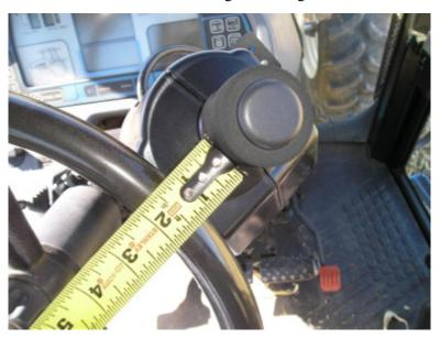
5. Pull the motor release knob. The motor will spring against the steering wheel.
