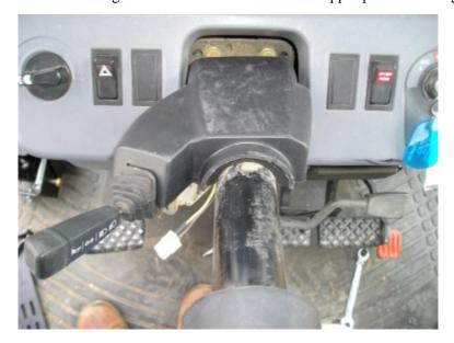
2. Tilt the steering column up and insert the ether switch into the lower housing.
