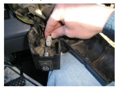
6. Remove the lower housing from around the steering column.
