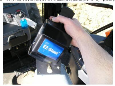
3. Install the motor drive onto the slotted arm bracket. Insert the carriage bolts and tighten the wing nuts that are included with the platform kit.
