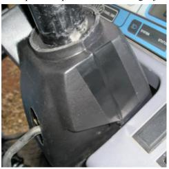
b. Apply a 2.5 cm (1 inch) long strip of tape to the top joint.
